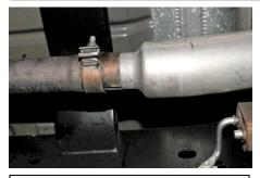
2. Install muffler assembly Item # A into the factory head pipe. You will re use the factory clamp at this connection. Install hanger into rubber grommet and loosely tighten down the clamp.
