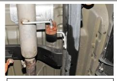
3. With the muffler assembly installed you may want to use a jack stand to support the muffler while installing the over axle pipe.
