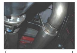
5. Install the Over axle pipe Item # C into the muffler outlet. With everything loose you may need to adjust the system for proper clearance of shocks, brake lines, ect.
