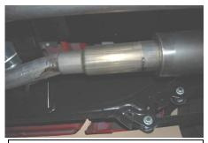
3. Install the muffler assembly Item # B onto the Head pipe Item # A. Slide the rear hangers into the factory rubber grommets.
