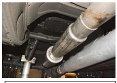
4. Install muffler assembly Item # B onto the head pipe. Use a jack stand to support the muffler while installing the tailpipe. Loosely tighten down the clamp.
