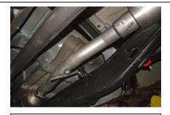
3. Use clamp Item # E to connect the muffler assembly to the headpipe.
