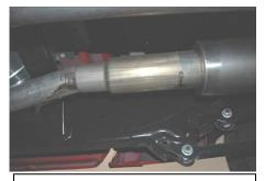
3. Install the muffler assembly Item # B onto the Head pipe Item # A. Slide the rear hangers into the factory rubber grommets.
