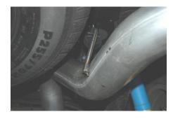
6. With proper clearance from the spare tire install the exhaust tip onto the tailpipe. The system was designed to have the tip 1" below the quarter panel of the vehicle. With the tip in your desired position begin to tighten down all clamp connections from the front head pipe back.
