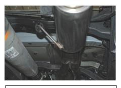
4. Be sure with the muffler supported by the hanger and installed on the head pipes that you keep everything loose to allow for final adjustments.
