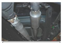
4. Install over axle pipe Item # C into the muffler outlet. Slip the hangers into the rubber grommets and keep tailpipe loose.
