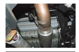
5. With everything loose you may need to adjust the system for proper clearance of shocks, brake lines, ect.
