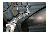
6. NEXT, USING TWO ZIP TIES SUPPLIED IN THE KIT, SECURE THE TWO BRAKE LINE HOSES AWARE FROM OVER AXLE PIPE. LINES MUST BE AT LEAST 1" FROM PIPE. THEN TAKE THE HEAT SLEEVE AND CUT IT LENGTHWISE IN ORDER TO WRAP AROUND BRAKELINES, SECURE WITH REMAINING 3 ZIP TIES.
