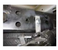
ON DRIVER SIDE: ATTACH REAR TAILPIPE HANGER #I TO FRAME USING BOLT KIT PROVIDED
