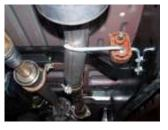
INSTALL HEADPIPE # A INTO STOCK FLANGE ATTACH WITH BOLT KIT PROVIDED. DO NOT TIGHTEN. INSERT WELDED HANGER INTO RUBBER GROMMET.
