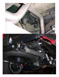
INSTALL PASSENGER SIDE TAILPIPE # C INTO MUFFLER 1½" TO 2". INSERT WELDED HANGER INTO RUBBER GROMMET, USE CLAMP # H TO SECURE PIPE TO MUFFLER. DO NOT TIGHTEN. ROTATE PIPE TOWARDS DRIVERSIDE.
