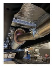
TO REMOVE YOUR STOCK EXHAUST, REMOVE IT FROM THE CLAMP LOCATED JUST IN FRONT OF THE RESONATOR. REMOVE HANGERS FROM RUBBER GROMMETS, USE WD-40 TO AID IN REMOVAL, LEAVE GROMMETS IN PLACE.
