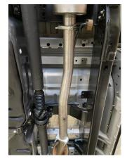
INSTALL HEADPIPE #A ONTO STOCK PIPE BEHIND RESONATOR. INSERT WELDED HANGER INTO RUBBER GROMMET. USE CLAMP #D PROVIDED TO SECURE. DO NOT TIGHTEN.
