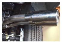
NEXT INSTALL DRIVERS OVER AXLE PIPE # D INTO MUFFLER 1½ TO 2".USE CLAMP # F TO SECURE PIPE TO MUFFLER. DO NOT TIGHTEN. USE BOLT KIT # H TO SECURE PIPES TOGETHER. DRIVERSIDE TAB WILL BE ON THE TOP
