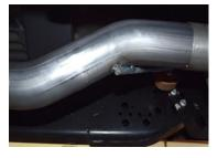
INSTALL HEADPIPE # A ONTO FACTORY PIPE. LINE UP THE NOTCH. USE CLAMP # G TO SECURE HEADPIPE TO FACTORY PIPE. DO NOT TIGHTEN. INSERT WELDED HANGER INTO RUBBER GROMMET.
