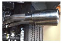
NEXT INSTALL DRIVERS OVER AXLE PIPE # D INTO MUFFLER 1½ TO 2".USE CLAMP # F TO SECURE PIPE TO MUFFLER. DO NOT TIGHTEN. USE BOLT KIT # H TO SECURE PIPES TOGETHER. DRIVERSIDE TAB WILL BE ON THE TOP
