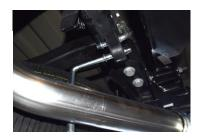
**6.** Install the driverside overaxle tailpipe #D into the muffler 1½-2". Use clamp #H to secure. DO NOT TIGHTEN. Rotate until it meets with the rubber grommet. DO NOT TIGHTEN.
