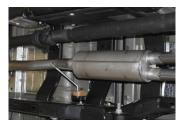
**3.** Install muffler #B onto head pipe #A 1½"-2" with the louvers facing towards the converter and muffler outlets level. Use a jack stand to support the muffler. Use clamp #G to secure the muffler to the headpipe. Do not tighten. Muffler inlet is looking into the louvers.
