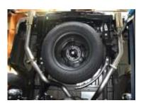
**7.** Next install the exit pipes #E. Use clamp #H to secure. DO NOT TIGHTEN. Rotate pipes to your desired look.
