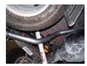
**6.** Install the driverside overaxle tailpipe #D into the muffler  $1\frac{1}{2}$ -2". Use clamp #H to secure. DO NOT TIGHTEN. Rotate until it meets with the rubber grommet. DO NOT TIGHTEN.
