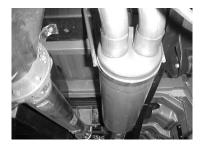
SLIP MUFFLER #B ONTO THE HEADPIPE 1 ½" TO 2". THE OUTLETS WILL BE LEVEL. USE CLAMP #G TO SECURE MUFFLER TO HEADPIPE. DO NOT TIGHTEN.
