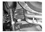
NEXT INSTALL DRIVERS OVER AXLE PIPE # D INTO MUFFLER 1½ TO 2".USE CLAMP # F TO SECURE PIPE TO MUFFLER. DO NOT TIGHTEN. USE BOLT KIT # H TO SECURE PIPES TOGETHER. DRIVERSIDE TAB WILL BE ON THE BOTTOM.
