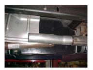
INSTALL HEADPIPE #A ONTO EXISTING PIPE. LINE UP THE NOTCH. USE CLAMP #H TO SECURE HEADPIPE TO STOCK PIPE. DO NOT TIGHTEN.
