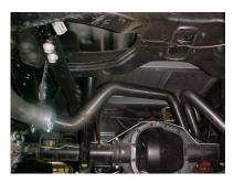
NEXT INSTALL DRIVERS SIDE OVERAXLE PIPE #D INTO MUFFLER 1 ½" TO 2". USE CLAMP #I TO SECURE PIPE TO MUFFLER. DO NOT TIGHTEN. ROTATE PIPE UNTIL IT TOUCHES HANGER. USE CLAMP #I TO HOLD PIPE TO HANGER DO NOT TIGHTEN.
