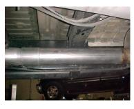
NEXT, INSTALL RESONATOR # B 1 ½"-2" ONTO Y-PIPE USE CLAMP # G TO SECURE PIPES TOGETHER, DO NOT TIGHTEN.
