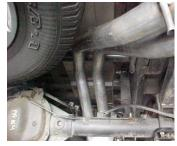
INSTALL PASS. SIDE TAILPIPE # E INTO MUFFLER 1 ½"-2". USE CLAMP # H TO SECURE PIPE TO MUFFLER, DO NOT TIGHTEN.
