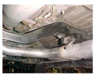
INSTALL Y-PIPE # A & L ONTO STOCK FLANGES USE YOUR STOCK HARDWARE TO SECURE INSERT WELDED HANGER INTO RUBBER GROMMET, DO NOT TIGHTEN. USE CLAMP #H TO SECURE PIPES TOGETHER. DO NOT TIGHTEN.
