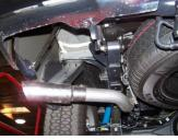
7. Install rear tailpipe hanger #K. Use bolt kit #L to secure. Use the hole on frame closest to the rear shackle. Install rubber grommet on rear hanger.
