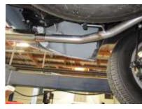
8. Install the exit pipes #E. Use clamp #H to secure exit pipes to tailpipes. DO NOT TIGHTEN. Rotate pipes to adjust for desired look. Reinstall spare tire.
