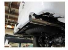
9. Install stainless steel tips #F. Clamp down. When you have everything in place and clear from all brake lines, shocks, etc. firmly tighten all bolts and clamps down securely beginning from the front. Inspect all fasteners after 25-50 miles of operation and re-tighten as necessary.
