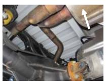
2. To remove the stock exhaust, remove it from the clamp in front of the muffler. Disengage the welded hangers using WD-40 from the OEM rubber grommets. Do not damage or remove the rubber grommets as you will reuse them to mount your new system.
