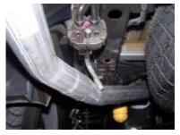
6. Remove spare tire to install tailpipes (Reference vehicle manual for removal of spare tire). Now install Driver side tailpipe #D into the muffler 11/2-2". Use clamp #H to secure tailpipe to muffler. DO NOT TIGHTEN. Insert welded hangers into rubber grommets.
