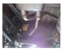
4. Install muffler #B onto head pipe #A 11/2"-2". Use a jack stand to support the muffler. Use clamp #G to secure the muffler to the headpipe. DO NOT TIGHTEN.
