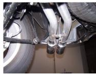
**9.** Install stainless steel tips #E. Clamp down. When you have everything in place and clear from all brake lines, shocks, etc. firmly tighten all bolts and clamps down securely beginning from the front. Inspect all fasteners after 25-50 miles of operation and re-tighten as necessary.
