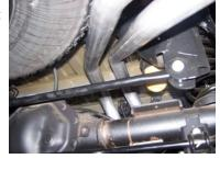
7. Install Driver side tailpipe #D into the muffler 11/2-2". Use clamp #G to secure tailpipe to muffler. DO NOT TIGHTEN. Insert welded hangers into rubber grommets. Use bolt kit # H to attach both tailpipes.
