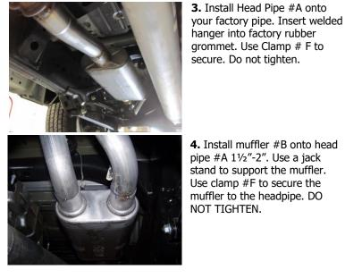
4. Install muffler #B onto head pipe #A  $1\frac{1}{2}$ "-2". Use a jack stand to support the muffler. Use clamp #F to secure the muffler to the headpipe. DO NOT TIGHTEN.
