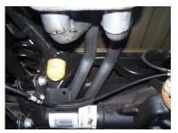
**6.** Install Passenger side tailpipe #C into the muffler  $1\frac{1}{2}-2^{\prime\prime}$ . Use clamp #G to secure tailpipe to muffler. DO NOT TIGHTEN. Insert welded hangers into rubber arommets.
