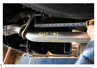
2) SECOND, CUT DRIVER SIDE OUTLET PIPE 6" FROM THE REAR LEAF SPRING BUCKET.
