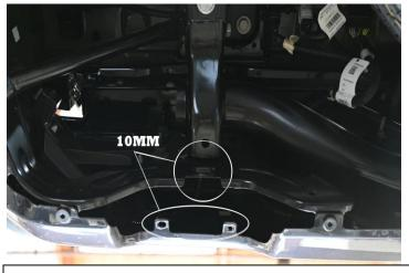
1) FIRST, REMOVE  $\underline{3}$  BOLTS HOLDING BOTH DRIVER AND PASSENGER SIDE FACTORY TIPS ON. THERE IS  $\underline{2}$  LOCATED ON THE INSIDE OF THE BUMPER AND 1 LOCATED DIRECTLY ABOVE THE TIP.
