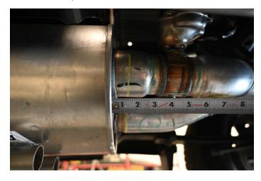
2) FIRST, CUT BOTH OUTLET PIPES 1.25" FROM THE FACE OF THE MUFFLER (NOT THE LIP).
