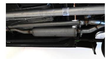
GIBSON EXHAUST systems are designed on a factory stock vehicle. Any aftermarket products installed could increase the sound levels of this Exhaust. Make sure there is a 1" clearance from ALL rubber brake lines, shock boots, fuel lines, tires, etc to prevent heat related damage or fire.
