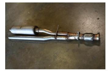
4) THEN, INSTALL HEADPIPE ONTO MUFFLER ASSY #A. ONCE INSTALLED YOU MAY INSTALL COMPLETE ASSEMBLEY INTO THE VEHICLE AND WELD ONCE ALL CLEARANCES HAVE BEEN CHECKED.
