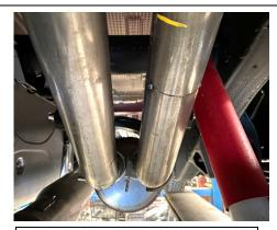
3. Install supplied 3½" clamp #H onto inlet end of new muffler #B and slip onto end of the head pipe with 2-1/4" inserted into muffler. Muffler outlets will sit level. Tighten with allowance for adjustment.
