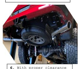
from spare tire, install the exhaust tip onto the tailpipe. The system was designed to have the tip 1" below the quarter panel of the vehicle. Note you can adjust the tip position inward or outward with rotation of the exit pipes.
