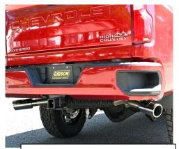
7.With a minimum of 1.5" clearance on all pipes begin to tighten down all clamp connections from the front head pipe back. Be sure to double check all clearance after your first heat cycle.
