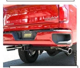
7.With a minimum of 1.5" clearance on all pipes begin to tighten down all clamp connections from the front head pipe back. Be sure to double check all clearance after your first heat cycle.
