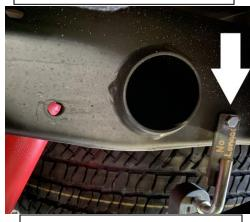
5. Install the Driver side hanger into the factory existing hole in frame. Install the Driver side pipes. Keep everything loose until everything is installed.
