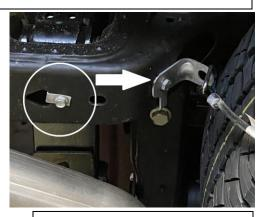
4. Relocate the the factory spare tire cable bracket to ten hole closer to the spare tire using bolt kit # L. You can install the passenger side overaxleipe. Note all hangers will sit in the rubber hangers level.
