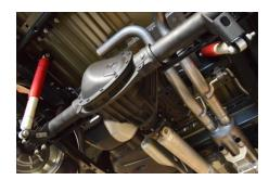
5. Install supplied 2-1/2" band clamp (Item I) onto the inlet side of the driver side overaxle pipe A(Item D)and install onto outlet of muffler. Install hanger into factory rubber grommet hanger. Next install another 2-1/2" band clamp(Item I) onto the inlet side of driver side over-axle pipe B(Item E) and install onto outlet of Item D. Tighten both clamps with allowance for adjustment.
