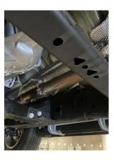
Install head pipe #A onto you're existing stock Pipe use your factory Band Clamp.
