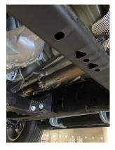
Install head pipe **#A** onto you're existing stock Pipe use your factory Band Clamp. Insert welded hanger into rubber grommet. Do not tighten.
