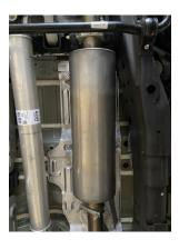
Install muffler onto head pipe #A 1-1/2" to 2" with the louvers facing towards the converter. Use a jack stand to support the muffler. Use clamp #H to the secure the muffler to the head pipe. Do not tighten
