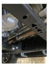
Install head pipe #A onto you're existing stock Pipe use your factory Band Clamp. Insert welded hanger into rubber grommet. Do not tighten.
