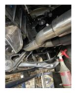
5. Finally, over axle pipe #C can be installed using the Band Clamp #D. Once the over axle pipe is in you may install Exit Pipe #E along with both Tips. (Tighten all clamps working from front to back.)
