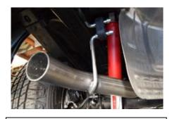
5. Before install of item E, install Driver side hanger bracket as shown in picture. Install supplied 2-1/2" band clamp onto the inlet side of the driver side over-axle pipe A and install onto outlet of muffler. Install hanger into factory rubber grommet hanger. Next install another 2-1/2" band clamp onto the inlet side of driver side over-axle pipe B(Item E) and install onto outlet of Item D. Tighten both clamps with allowance for adjustment.
