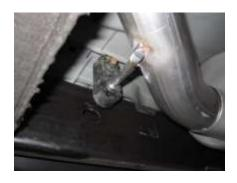
6.Next install passenger side tailpipe # D into muffler 1.5"to 2" insert welded hangers into rubber grommets use clamp #F to secure pipe together do not tighten
