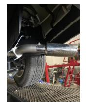
Re install spare tire and heat shield. Position all pipes and double check all connections prior to tightening clamps.
