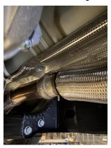
TO REMOVE YOUR STOCK EXHAUST, Un Bolt the back half from the flange LOCATED above the rear suspension, then loosen the front clamp and remove the remaining exhaust. Your Spare Tire & Heat Shield will need to be removed for installation. (FACTORY **RUBBER HANGER GROMMETS WILL BE RE-**USED, USE WD-40 TO AID IN **REMOVAL.)**
