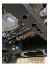
Install head pipe #A onto you're existing stock Pipe use your factory Band Insert welded hanger into rubber grommet. Do not tighten.
