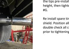
Re install spare tire and heat shield. Position all pipes and double check all connections prior to tightening clamps.
