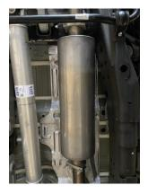
Install muffler onto head pipe **#A** 1-1/2" to 2" with the louvers facing towards the converter. Use a jack stand to support the muffler. Use clamp #H to the secure the muffler to the head pipe. Do not tighten
