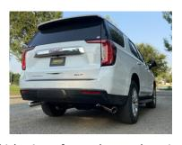
Finally, go back and tighten all clamps, nuts and bolts. Use stainless steel cleaner and a Scotch Brite pad weekly to prevent tip from discoloration. Inspect all fasteners after 25-50 miles of operation and retighten as necessary.
