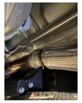
TO REMOVE YOUR STOCK EXHAUST, Un Bolt the back half from the flange LOCATED above the rear suspension, then loosen the front clamp and remove the remaining exhaust. Your **Spare Tire & Heat Shield** will need to be removed for installation. (FACTORY RUBBER HANGER GROMMETS WILL BE RE-USED, USE WD-40 TO AID IN REMOVAL.)
