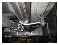
3. Next, install headpipe #A into the factory pipe. Insert welded hanger into the rubber grommet. Do not tighten
