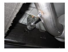
6.Next install passenger side tailpipe # D into muffler 1.5"to 2" insert welded hangers into rubber grommets use clamp #F to secure pipe together do not tighten.
