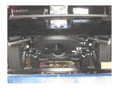
7. Install exit pipes #E onto tailpipes use clamp # F to secure together. Next, install tips onto exit pipes.
