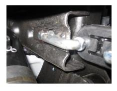
5. Next install drivers side rear hanger and grommet with bolt kit provided. See picture the hanger goes on the outside of the frame and bolts through the first wall of the frame.
