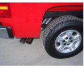
8. Install stainless steel tip. Clamp down. When you have everything in place, firmly tighten all bolts and clamps down securely. Use stainless steel cleaner weekly to prevent tip from discoloration. Inspect all fasteners after 25-50 miles of operation and re-tighten as necessary.
