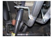
5. Make sure muffler outlets are level before installing tailpipes. Now install passenger tailpipe #C. Insert welded hangers into rubber grommets.
