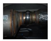
2. To remove stock exhaust, unclamp it at the ball flange behind the Y-pipe. Make sure to leave all rubber grommets in the factory location. **You will re-use stock clamp.** For easier removal of exhaust, cut behind the muffler. Use WD-40 to remove hangers from grommets.
