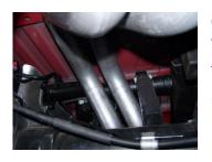
6. Slide the driver side over axle tailpipe #D into the muffler 1.5-2". Use clamp #G to secure tailpipe to muffler. Do not tighten. Insert welded hanger into rubber grommet.
