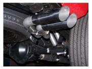
7. Use bolt kit #h to attach tailpipe tabs together.
