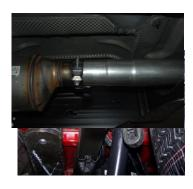
5. Install metal hanger #H into hole located approximately 16" from the rear of the frame. Use hardware kit #I, washer #M, and rubber grommet #J.
