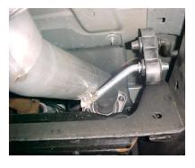
INSTALL HEAD PIPE # A ONTO YOUR EXISTING STOCK FRONT PIPE. INSERT WELDED HANGER INTO RUBBER GROMMET.
