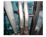
Install driverside headpipe #B. Then install headpipe #A and insert welded hanger into rubber grommet. Secure both pipes with clamp #G. Do not tighten.
