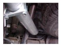
INSTALL DRIVER SIDE TAILPIPE #D INTO MUFFLER AT LEAST 1½" TO 2". THIS PIPE WILL ROUTE OVER THE AXLE AND BETWEEN THE SHOCK AND TIRE. ATTACH CLAMP #G TO SECURE TAILPIPE TO MUFFLER. DO NOT TIGHTEN. INSERT WELDED HANGER INTO RUBBER GROMMET.
