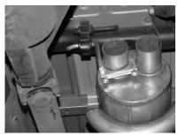
INSTALL EXIT PIPES #E ONTO TAILPIPES AND ATTACH TO HANGER #H AND CLAMP #G TO SECURE EXIT PIPES TO TAILPIPES. THESE METAL HANGERS NEED TO BE ROTATED IN ORDER TO ADJUST FOR CLAMPING. CUT TO YOUR PREFERED LENGTH. NOW INSTALL YOUR STAINLESS STEEL TIPS TO YOUR DESIRED LOOK. NOW YOU CAN TIGHTEN ALL CLAMPS, NUTS, AND BOLTS. STARTING FROM THE FRONT WORKING BACK. USE ZIP TIES TO TIE AWAY BRAKE LINES.
