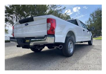
GIBSON EXHAUST systems are designed on a factory stock vehicle. Any aftermarket products installed could increase the sound levels of this Exhaust. Make sure there is a 1" clearance from ALL rubber brake lines, shock boots, fuel lines, tires, etc to prevent heat related damage or fire.
