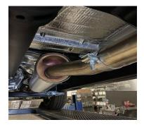
**2.** To remove the stock exhaust loosen the clamp from the back of the resonator. Then remove the spare tire and heat shield to aid in removal. Disengage the welded hanger using WD-40 from the OEM rubber grommets. Do not damage or remove the rubber grommets as you will reuse it to mount your new system.
