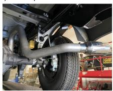
**5.** Now you may install the Over Axle Pipe #B into the muffler using Clamp #C. Then install the Tip onto the over axle to your desired location and tighten all clamps working front to back.
