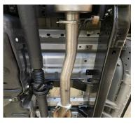
**3.** Install Head Pipe pipe #A onto your existing stock pipe coming out of the Resonator and attach with clamp # C. Keep the clamp a little loose.
