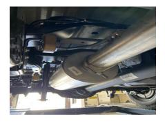
**4.** Install the Muffler #D onto the new Head Pipe using clamp #C. Leave clamps loose enough to have a little play.
