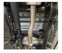
**3.** Install Head Pipe pipe #A onto your existing stock pipe coming out of the Resonator and attach with clamp # C. Keep the clamp a little loose.
